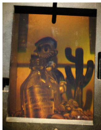
Fig. 5. Contour fringes obtained when a diode laser was used.
