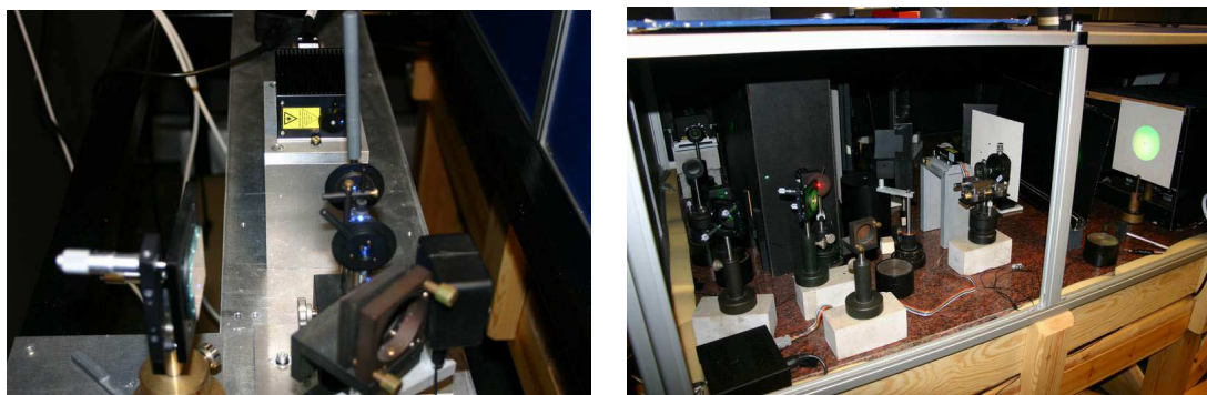
Fig. 2. Pictures of the holographic system. The blue Cobalt laser at the left is outside the table.
