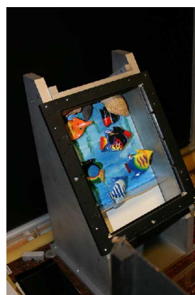
Fig. 6. Plate holder for 20 × 25 plates. The object is mounted upside down.
